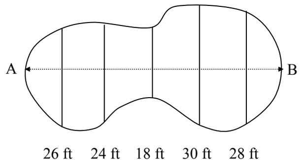
Step 4. Add the lengths of all of the offset lines and multiply by the distance between the offset lines.
