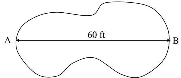
Step 2. Mark offset lines at right angles to the longest line. Choose the number of offset lines so that they divide the length line into equal parts. Tip: The closer the offset lines are to one another, the more accurate the estimation of the square footage.
